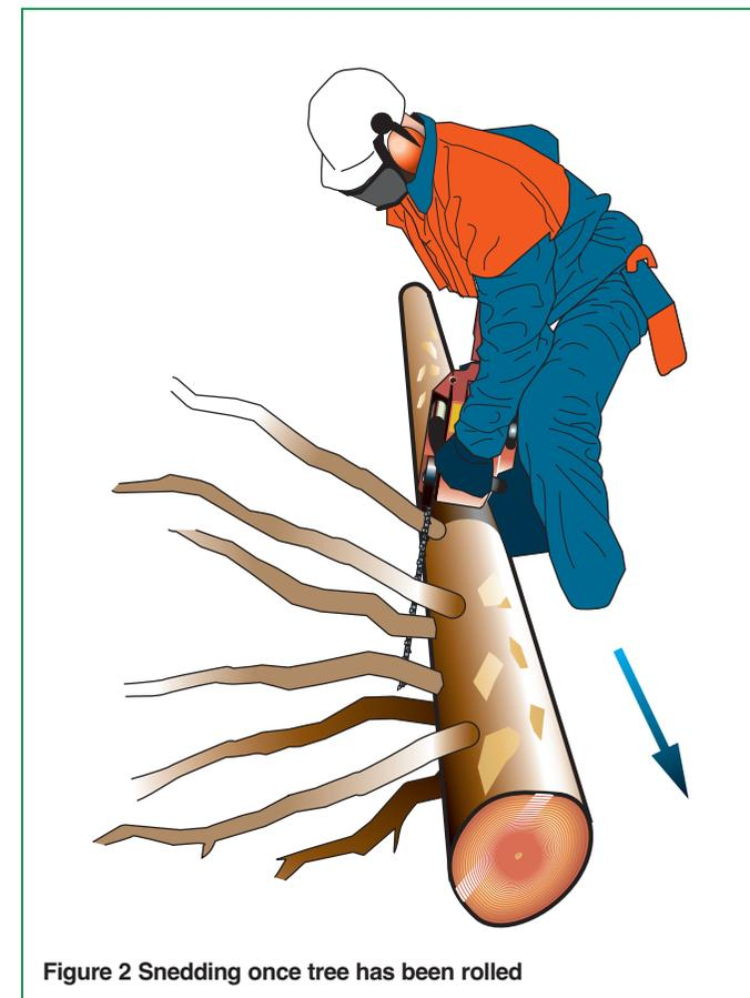
Figure 2 Snedding once tree has been rolled
